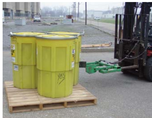
Drums of waste are loaded onto a pallet for shipment.
