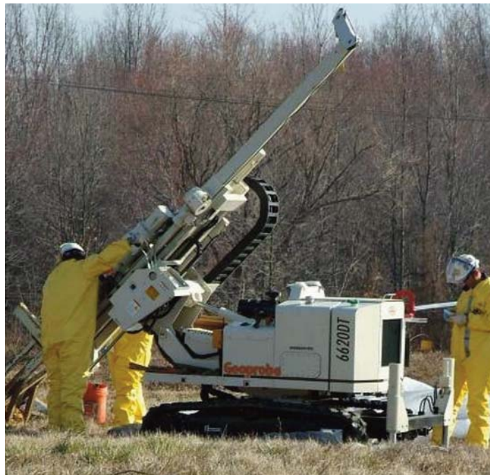
A sample boring is taken during the Burial Grounds Operable Unit Remedial Investigation.
